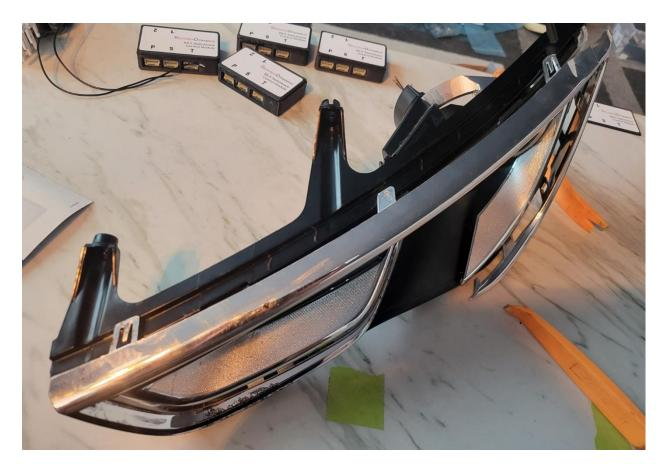
Next you can remove this trim, by prying in this final location. There are several tabs in this location, so it can be difficult to remove this section. After that the top light tube can be removed relatively easily.
